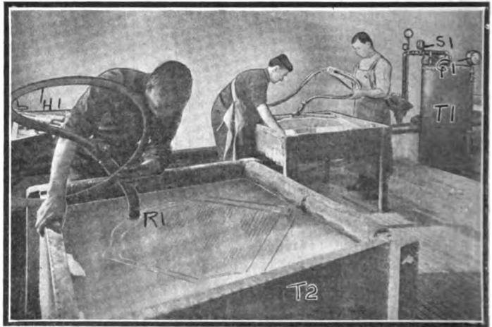
Fig. 13—Testing radiators by compressed air to locate leaks and to prove mechanical strength
